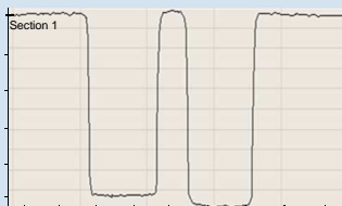
Individual NanoCD line feature (top) and the corresponding average profile (bottom) measured with a MCNT-500™.
